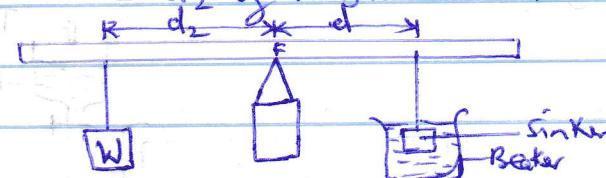
Using moments and letting,  $W'_s = \text{weight of sinker in water}$
