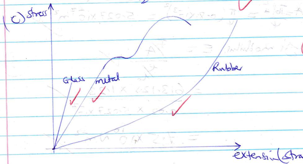
Metal - metal undergoes both elastic and plastic deformation. Before reaching the proportional limit, the stress is directly proportional to the strain.
