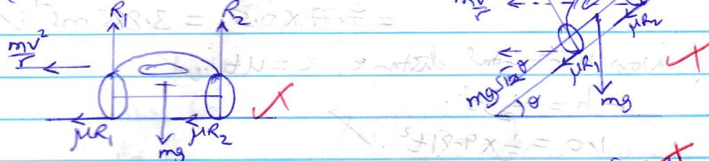
On a flat track, the centripetal force is provided for by only the frictional force. Thus  $\frac{mv^2}{r} = \mu(R_1 + R_2)$  X (i).
