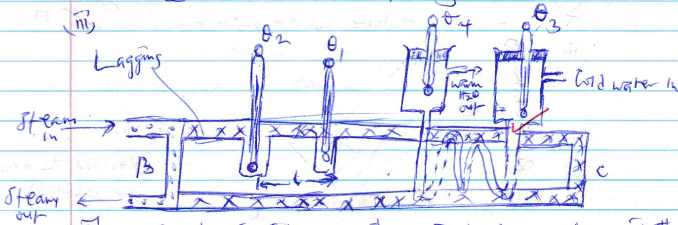
The apparatus is set up as shown in the figure above, with the specimen metal rod  $AB$  long compared to its diameter.
